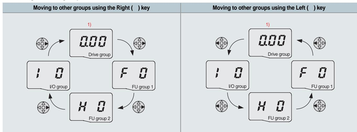
1) Target frequency can be set at 0.0 (the 1st code of drive group). Even though the preset value is 0.0, it is user-settable.
