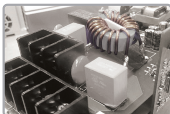
Built-in EMC Filter (C2 class)
