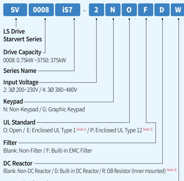
Note 1) For 0.75~75kW range, enclosed type 1 can be satisfied if conduit option installed.
