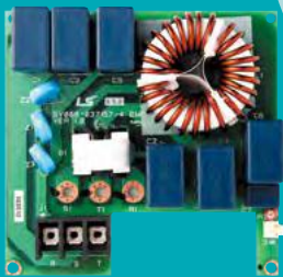
EMC Filter (In Conformity With EN61800-3) Built-in For Protection From Excessive Electronic Distortion
