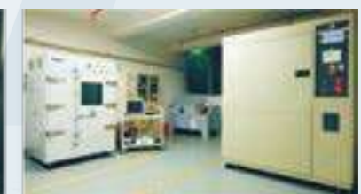
Natural Convection Test Chamber (L) Thermal Shock Test Chamber (R)
