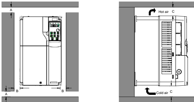
Figure 4-3 Installing one VFD
